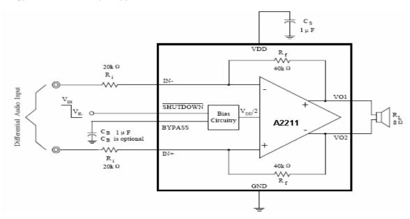
2. Differential Input application with Input Capacitors
